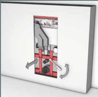
After removal of the bare-wall protection, the support for the lower glass facing is adapted to the wall thickness. The depth is adjusted by means of two adjusting nuts in the frame.
