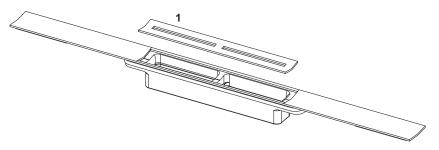
1 675000 Profiled cover in stainless steel, brushed 675001 Profiled cover in stainless steel, polished
